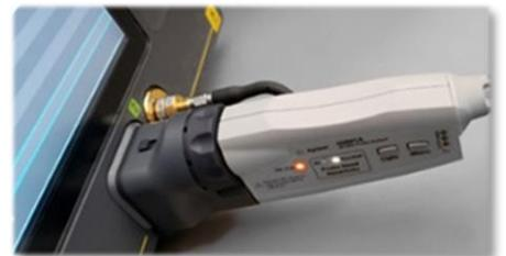
**AutoProbe II to AutoProbe III interface adapter**
