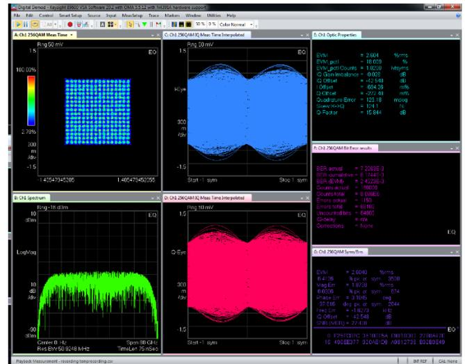
Never before seen 64 Gbaud 256 QAM 1-Tb/s coherent modulation analysis with 2.6% EVM – made possible by the Infiniium UXR-Series real-time oscilloscope and its world's lowest noise, 110 GHz of bandwidth, 256 GSa/s sampling, high-definition 10-bit ADC and industry best ENOB
