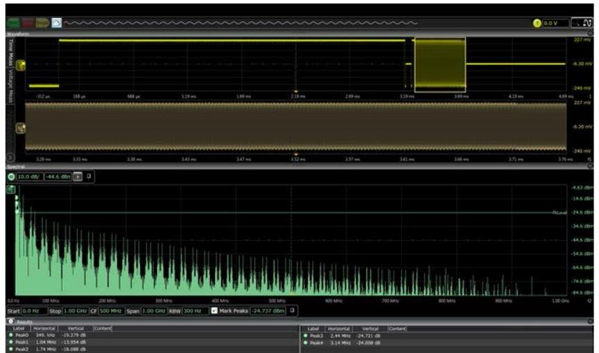
The UXR-Series FFT quickly identifies peaks and has key controls such as span, start and stop, which make the oscilloscope behave more like a spectrum analyzer
