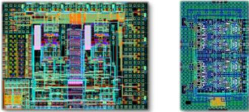
Keysight utilizes a proprietary Indium Phosphide (InP) integrated circuit process to design the key technology blocks necessary to deliver high-bandwidth performance, ultra-low noise and high-voltage signal input. This process is used in the pre-amplifier, trigger, sampling, and probe amplifier integrated circuit designs. Not only does this mean you are purchasing the best oscilloscope on the market today, but you can also count on technology leadership from Keysight in the future.
