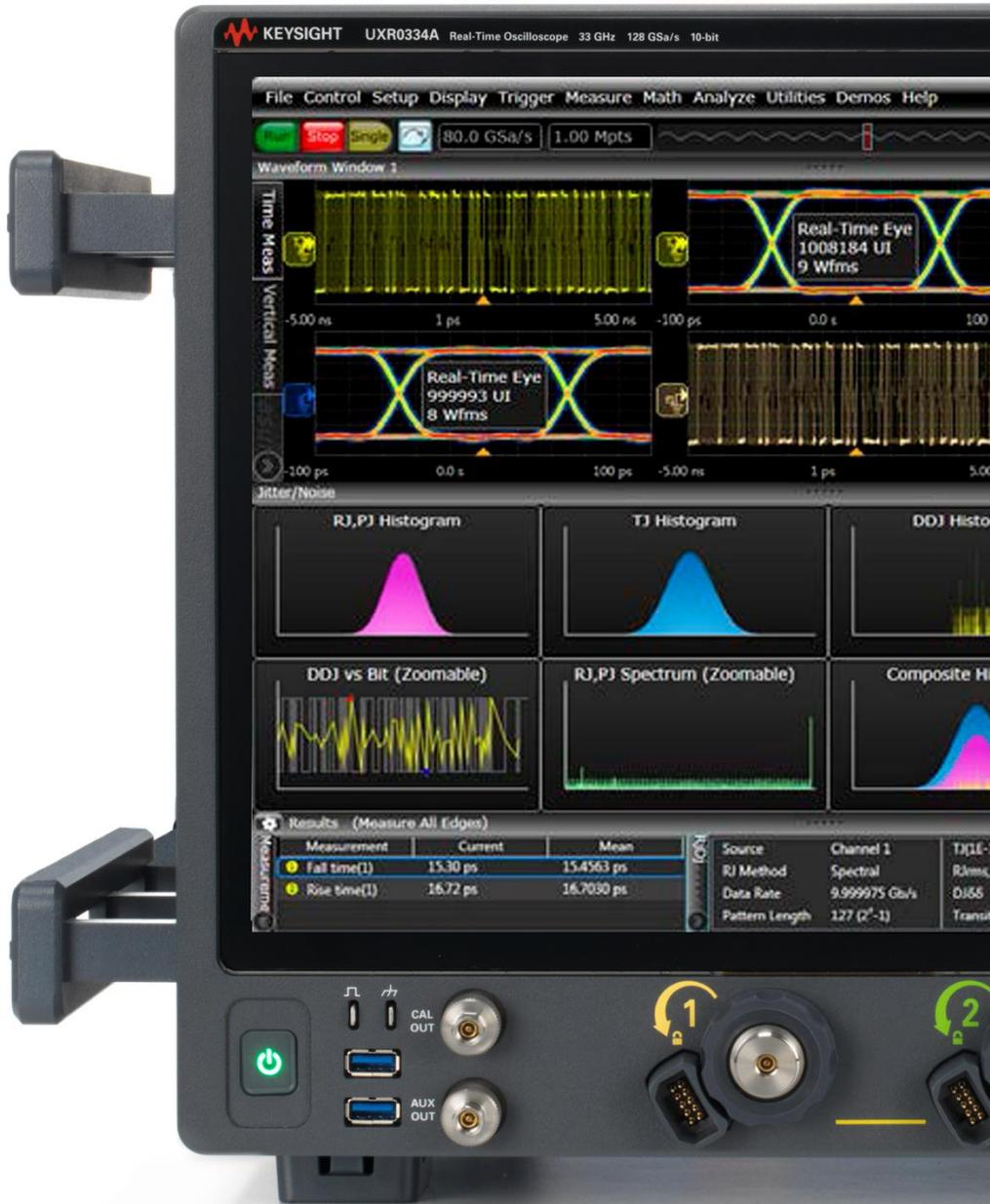
Threaded 3.5 mm RF connectors with convenient auto torque mechanism ensures the most reliable signal integrity and consistent 8 in-lbs connection. The AutoProbe II interface provides a robust interface and instant compatibility with the InfiniiMax III and III+ probing system.
